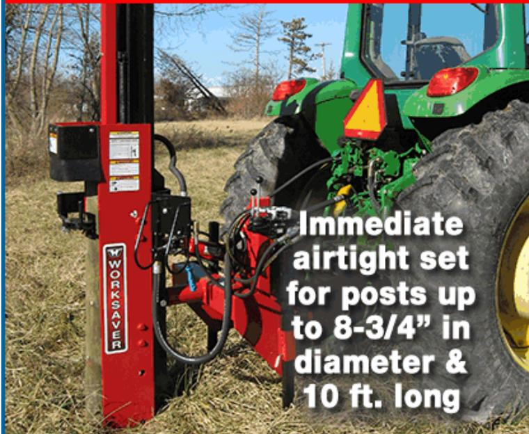
Immediate airtight set for posts up to 8-3/4" in diameter & 10 ft. long
